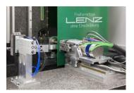
Traditional drilling and routing style programs are used to operate the machine. Both spindles, the tool selection, all depth control requirements and all drilling and routing are controlled by a single CNC program. The SLG greatly reduces Final Fab processing time as all functions are performed sequentially in a single setup and cycle. The engineered process approach eliminates the dependence on key operators to perform these more challenging machining functions.
