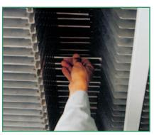
The magazine holds up to 20 PCB stacks, and is attached to the back of the drilling machine whilst remaining freely accessible.
