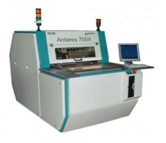
Manual panel load to the machine table - Panel alignment with reference to laser lines - rear auto unloader with cart for worked panels- scrap panels are re-presented to operator for unloading – Turbine spindle 30 Krpm – Pneumatic Z-Axis.
