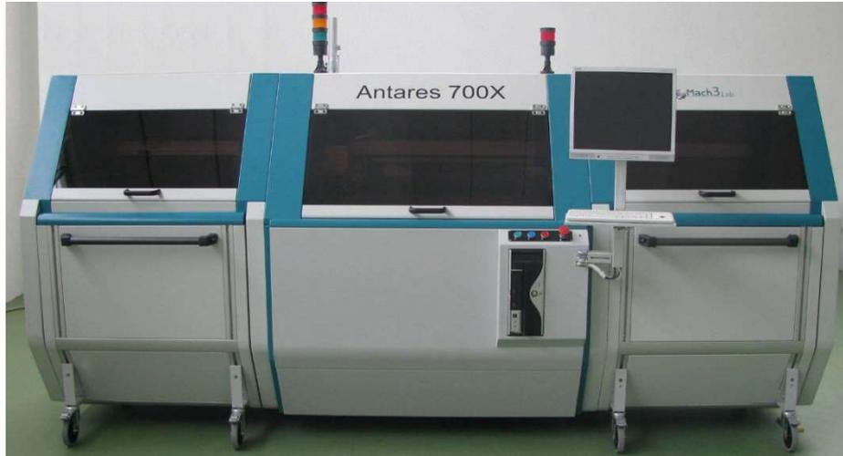
Automatic pick up from input cart where panel must be stacked (at left) – Automatic lay down of worked panels to the output cart (at right) – Turbine spindle 30 Krpm – Pneumatic Z-axis – Rear cart for auto unload of scrap panels.
