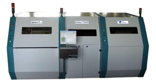
A line able to process Multilayer boards after the press cycle and before the drilling process.
