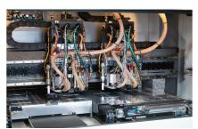
spindle and one high torque drill/rout spindle is mounted on each work station.
