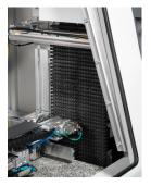
An anti-vibration belt and self sufficient mounting ensures the safe handling of the machine's tools. The belt holds over 5300 tools. Refilling of the tools can be carried out during production runs, thereby reducing downtime. The refilling station is ergonomically posited underneath the user interface.
